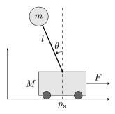
The state consists of the horizontal position of the cart center  $p_x$ , the angle of the pendulum  $\theta$ , as well as the respective velocities  $v_x$  and  $\omega$ . The pendulum has length l with a mass m mounted at its tip. The cart has mass M and can be actuated by applying a horizontal force F, i.e., u = F. The corresponding dynamics are
