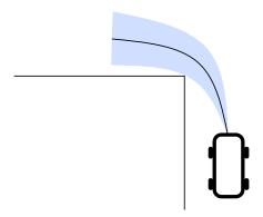
Due to uncertainty, the center of the tube needs to keep a distance ("backoff") from the corner.
