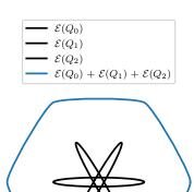
The sum of ellipsoids is not ellipsoidal.
