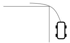
The predicted trajectory cuts the corner tightly, in *nominal MPC*.
