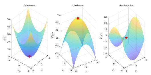
a stationary point w with  $\nabla F(w)=0$  can be a minimizer, a maximizer, or a saddle point
