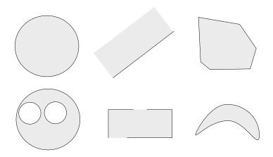
A set  $\Omega$  is said to be convex if for any  $w_1,w_2$  and any  $\theta\in[0,1]$  it holds  $\theta w_1+(1-\theta)w_2\in\Omega$  Figure inspired by Figure 2.2 in S. Boyd and L. Vandenberghe. Convex optimization. Cambridge university press, 2004.
