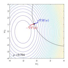
Ball rolling down a valley blocked by a fence - test problem with two variables and one inequality constraint
