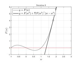
To solve a nonlinear system, solve a sequence of linear systems
