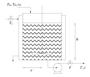
An irreversible, first-order reaction  $A \to B$  occurs in the liquid phase and the reactor temperature is regulated with external cooling. Mass and energy balances lead to the following nonlinear model:
