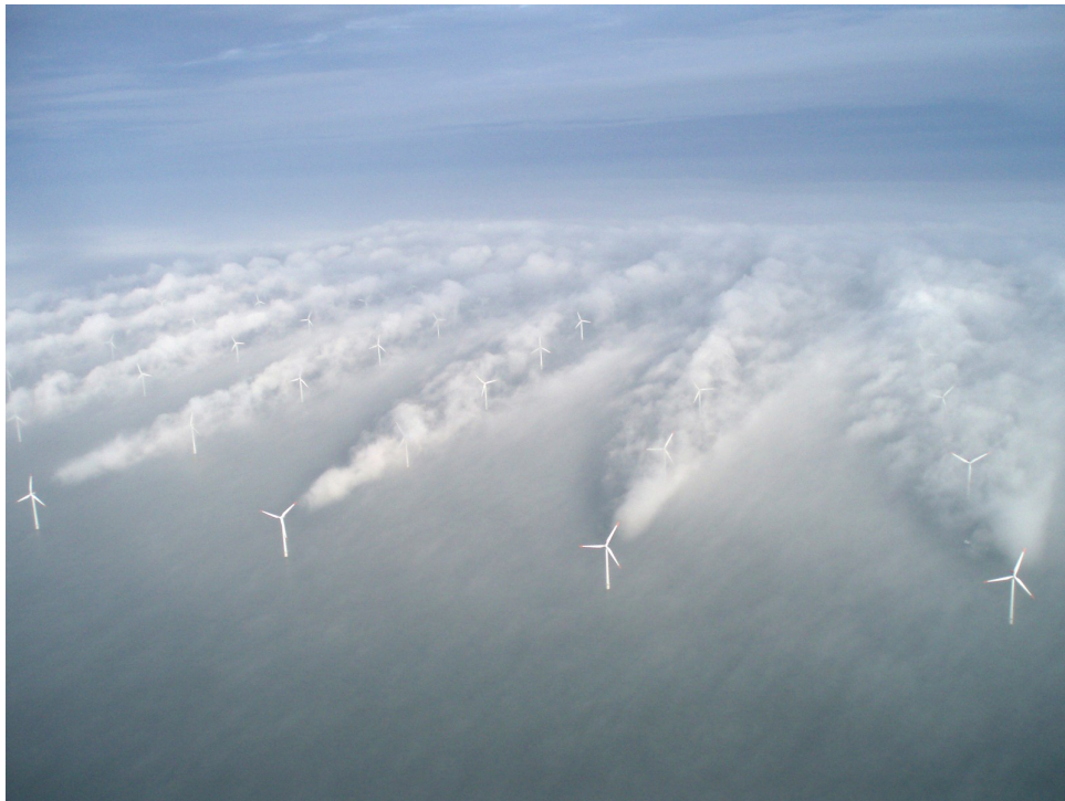
Figure 3.1: Photo of wakes forming behind turbines in a wind park. Source: Vattenfall.
