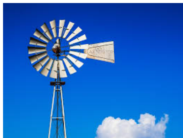
Figure 5.2: Vane used for passive orientation of a wind turbine.
