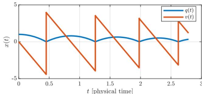
Phase plot of bouncing ball trajectory:
