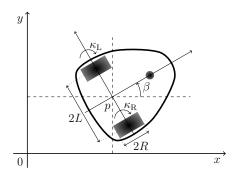
We model the robot's state  $x \in \mathbb{R}^5$  by  $x = [p_1, p_2, \beta, v, \omega]^{\top}$  where  $p = (p_1, p_2) \in \mathbb{R}^2$  denotes the position of the robot in m,  $\beta \in [0, 2\pi]$  denotes its orientation in rad,  $v \in \mathbb{R}$  denotes its forward velocity in  $\frac{m}{s}$ , and  $\omega \in \mathbb{R}$  denotes the angular velocity in  $\frac{rad}{s}$ . Note that we omitted the time dependence for cleaner notation, i.e. x = x(t). The time derivatives are given by
