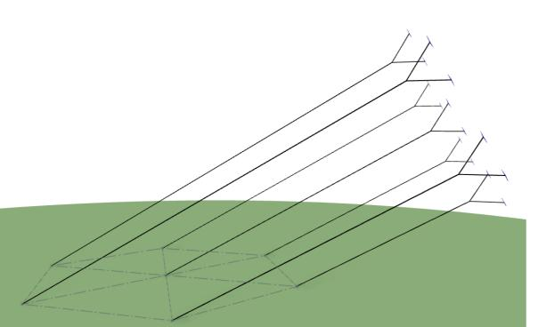
30 MW/km<sup>2</sup> for "Vertical Wind Farm" consisting of dual kite systems in varying altitudes (estimate by M.D.)
