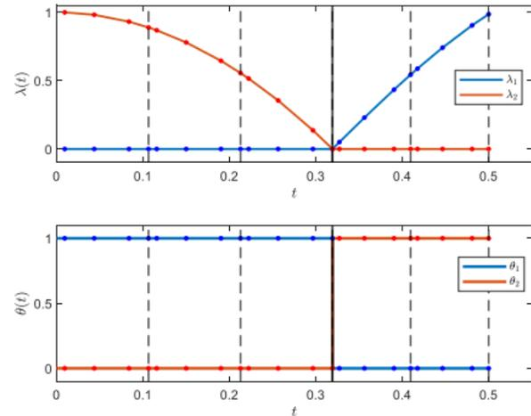
FESD's cross-complementarities exploit the fact that the multiplier  $\lambda_i(t)$  is continuous in time. On boundary,  $\lambda_i(t_k)$  must be zero if  $\theta_i(t) > 0$  for any  $t \in [t_{k-1}, t_{k+1}]$  on the adjacent intervals.
