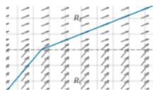
**NSD2:** state dependent ("internal") switch of RHS, e.g.  $\dot{x} = 2 - \text{sign}(x)$
