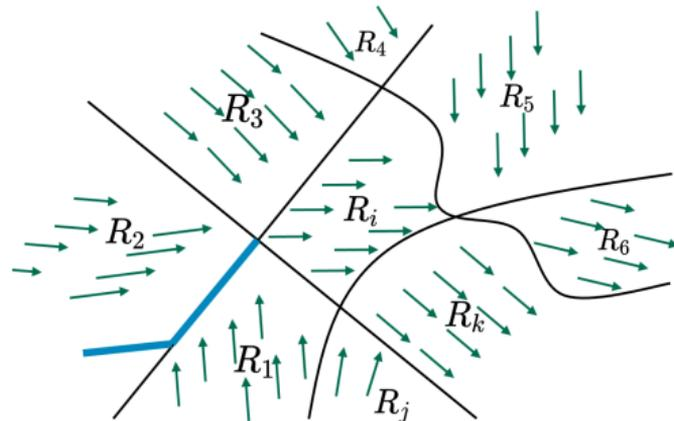
Dynamics not yet well-defined on region boundaries  $\partial R_i$ . Idea by A.F. Filippov (1923-2006): replace ODE by differential inclusion, using convex combination of neighboring vector fields.
