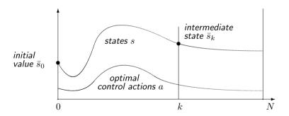
Subarc on [k, N] is optimal solution for initial value  $\bar{s}_k$ .
