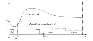
Use numerical integration to obtain state as function x(t; q) of finitely many control parameters  $q = (q_0, q_1, \dots, q_{N-1})$
