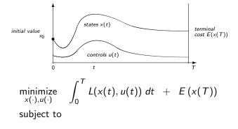
$\begin{aligned} x(0)-x_0 &= 0, \qquad \qquad (\text{fixed initial value})\\ \dot{x}(t)-f(x(t),u(t)) &= 0, \qquad t \in [0,T], \quad (\text{ODE model}) \end{aligned}$
