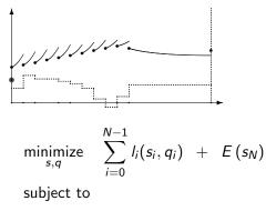
$$\begin{split} s_0 - x_0 &= 0, & \text{(initial value)} \\ s_{i+1} - x_i(t_{i+1}; s_i, q_i) &= 0, \ i = 0, \dots, N-1, & \text{(continuity)} \\ h(s_i, q_i) &\geq 0, \ i = 0, \dots, N, & \text{(discretized path constraints)} \\ r(s_N) &\geq 0. & \text{(terminal constraints)} \end{split}$$
