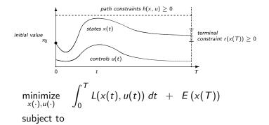
$$\begin{aligned} x(0) - x_0 &= 0, & (\text{fixed initial value}) \\ \dot{x}(t) - f(x(t), u(t)) &= 0, & t \in [0, T], & (\text{ODE model}) \\ h(x(t), u(t)) &\geq 0, & t \in [0, T], & (\text{path constraints}) \\ r(x(T)) &\geq 0 & (\text{terminal constraints}) \end{aligned}$$
