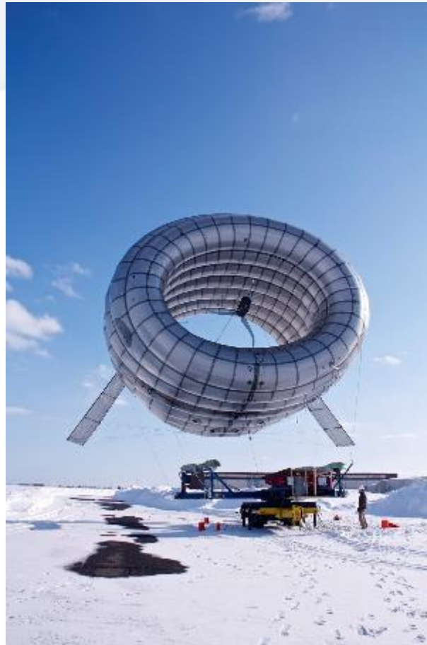
Altaeros: 20 kW commercial prototype system
