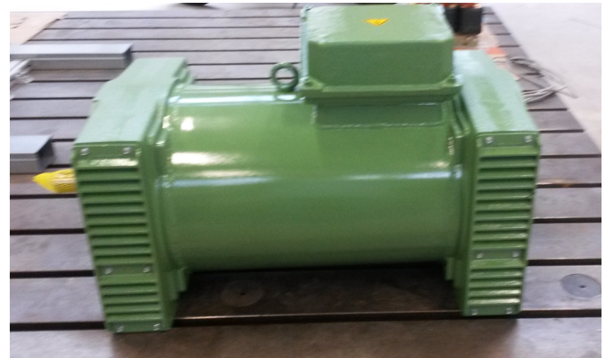
E lectrically E xcited S ynchronous M achine (EESM) 10 kW, 64Nm, 1500 RPM, 3 \phi , 400 V
