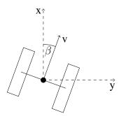
The system can be described by a state space model with three internal states. The state vector  $\mathbf{x} = [x \ y \ \beta]^{\top}$  contains the position of the robot in the X-Y plane and the deviation  $\beta$  from its initial orientation. The system can be controlled by the angular velocities of the wheels:  $\mathbf{u} = [\omega_L \ \omega_R]^{\top}$ . The output of the system is the position of the robot:  $\mathbf{y} = [x \ y]^{\top}$ . The model follows as
