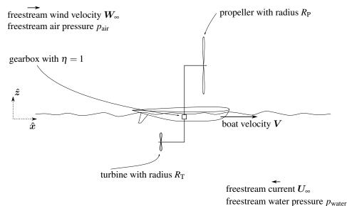
Assume a constant water density  $\rho_{water}$  and air density  $\rho_{air}$ , and that the boat is travelling parllel to both the uniform freestream wind velocity W, the uniform freestream current U, and  $\hat{x}$  which is perpendicular to the acceleration of gravity.
