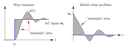
For a good controller performance, one would demand for a fast response and little overshooting, hence for minimizing the shaded areas. The performance index for the LQR controller is introduced as
