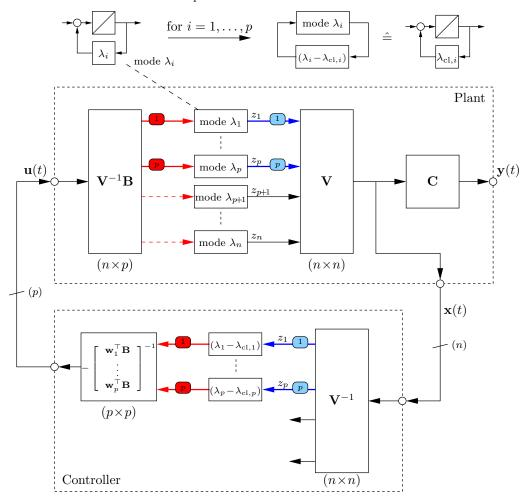
The controller 'picks out' the first p eigenmodes and 'shifts them towards' the desired values  $\lambda_{\text{cl},1},\ldots,\lambda_{\text{cl},p}$ . Note that a coupling to the remaining modes is introduced as indicated by the red dashed arrows. However, the coupling does not modify the other eigenvalues  $\lambda_{p+1},\ldots,\lambda_n$ .
