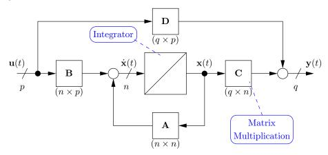
**SISO and MIMO systems** In a LTI system, the state vector  $\mathbf{x} \in \mathbb{R}^n$  has dimension n, the input vector  $\mathbf{u} \in \mathbb{R}^p$  has dimension p and the output vector  $\mathbf{y} \in \mathbb{R}^q$  had dimension q. Therefore, the state space matrices have dimension:  $\mathbf{A} \in \mathbb{R}^{n \times n}$ ,  $\mathbf{B} \in \mathbb{R}^{n \times p}$ ,  $\mathbf{C} \in \mathbb{R}^{q \times n}$  and  $\mathbf{D} \in \mathbb{R}^{q \times p}$ .
