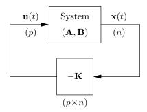
For SISO systems the feedback matrix **K** has the dimensions  $(1 \times n)$  and is determined uniquely by given n eigenvalues. For MIMO system there is an ambiguity and an infinite number of possible feedback realizations for n given eigenvalues. Hence, different controller design principles have to be applied.
