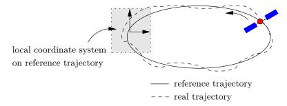
In absence of disturbances and with zero steering input, the satellite would fly on the orbit, denoted as solid trajectory. By introduction of a local (orthogonal) coordinate system, we only consider deviations from this reference trajectory.  $\mathbf{x} = \mathbf{0}$  would then describe a satellite flying on the reference trajectory. As deviations are expected to be small compared to the overall trajectory, linearization of the spherical coordinate system is an adequate modelling approach.
