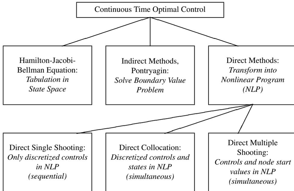
Figure 8.2: The optimal control family tree.
