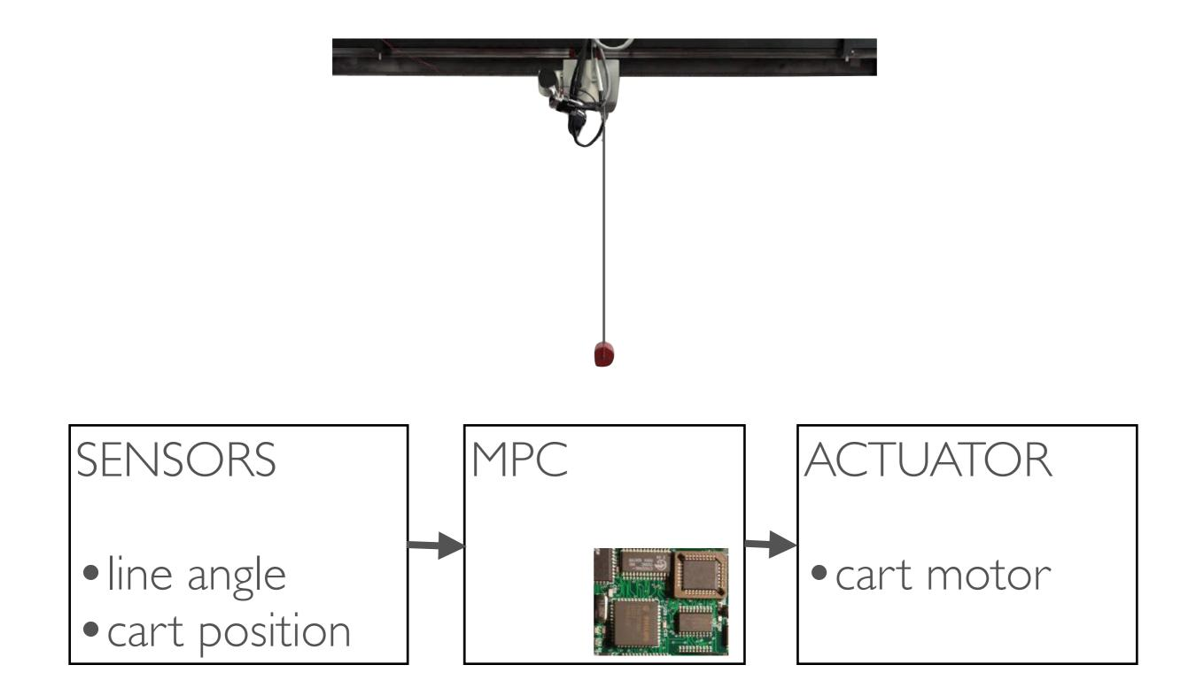
Hardware: xPC Target. Software: qpOASES [Ferreau, D., Bock, 2008]
