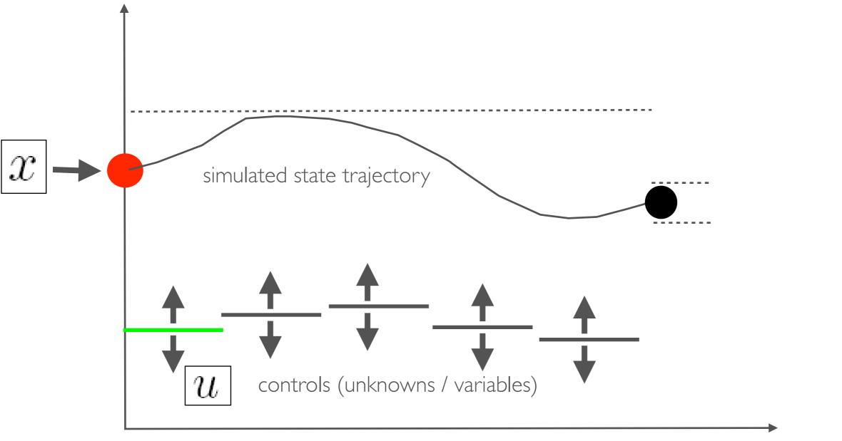
prediction horizon (length also unknown for time optimal MPC)
