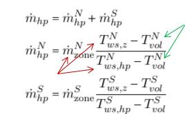
$$T_{wr,hp} = \frac{\dot{m}_{hp}^S}{\dot{m}_{hp}} T_{vol}^S + \frac{\dot{m}_{hp}^N}{\dot{m}_{hp}} T_{vol}^N$$
